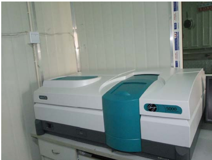
Transmission testing for deep OD(up to OD6)
