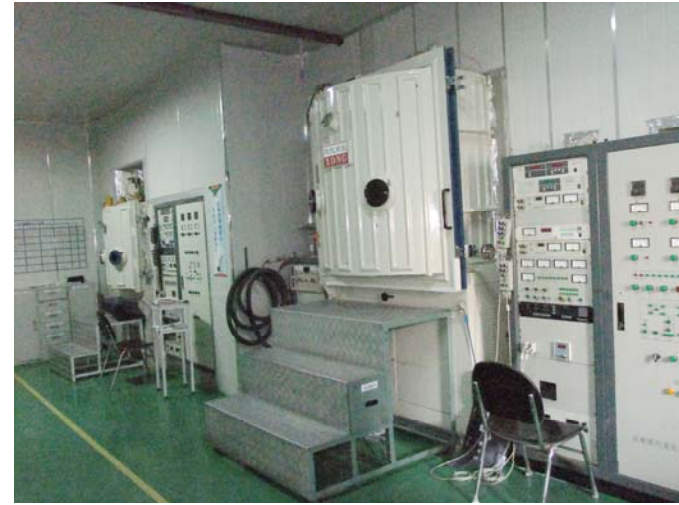
Coaters, 900mm and 1300mm chamber IAD E-beam evaporation
